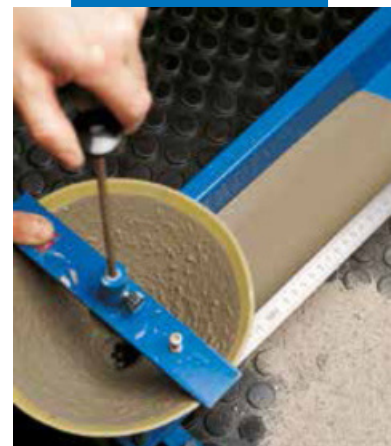
Flow test according to the Italian norm UNI 8997/89
