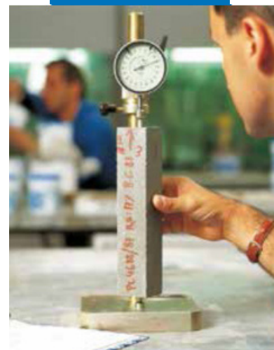
Measuring restrained expansion according to the Italian norm UNI 8997/89
