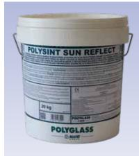
**POLYSINT SUN REFLECT** is a water-based fibre-reinforced acrylic liquid membrane in white, offering high solar reflectivity and thermal emissivity ratings (83% and 91% respectively), with a solar reflectance index (SRI) of 105, for protecting bitumen waterproofing membranes and concrete surfaces.
